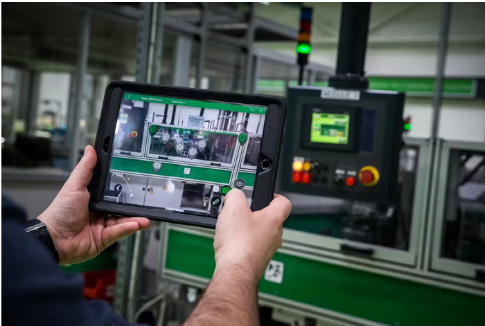
Augmented reality operator assist software deployed at the Lexington plant displays machine information over a mobile device's camera view.
